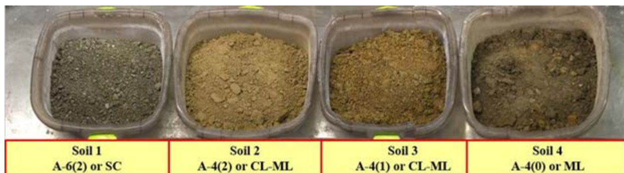
Figure 10. Collected four types of soil in Iowa for research
