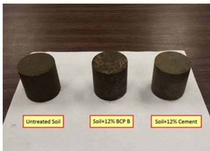
Figure 17. Prepared 2 in. by 2 in. samples
