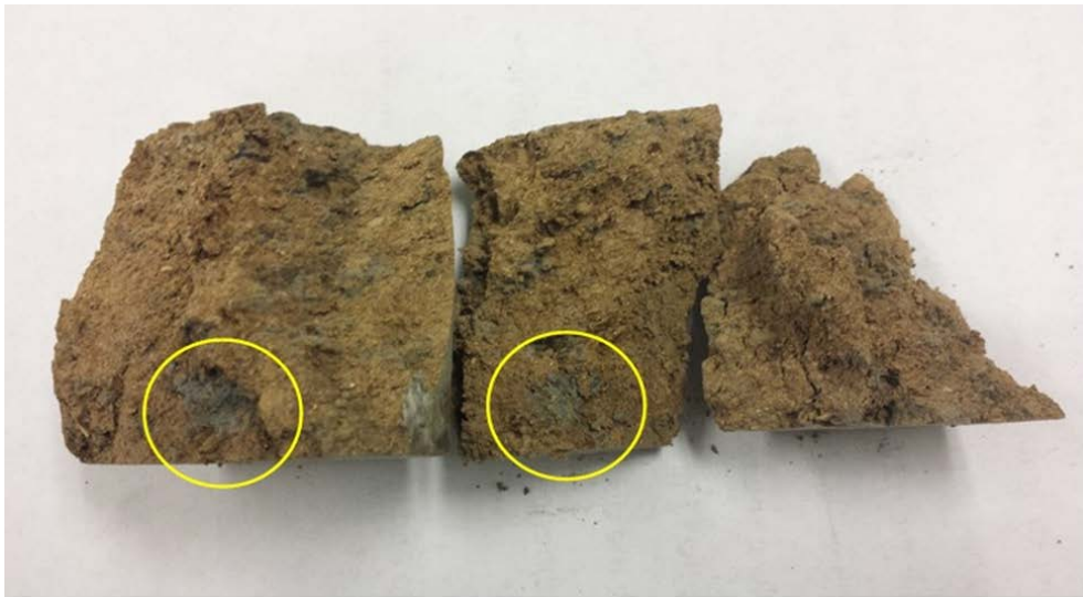
Figure 43. Bacterial colony in BCP B-treated specimen
